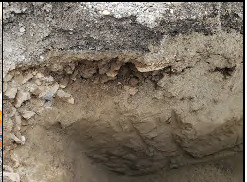
Exposed subsurface soil profile to ~9' BGS within test pit P-2
