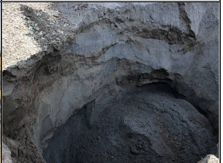
Exposed soil profile within test-pit TP-6
