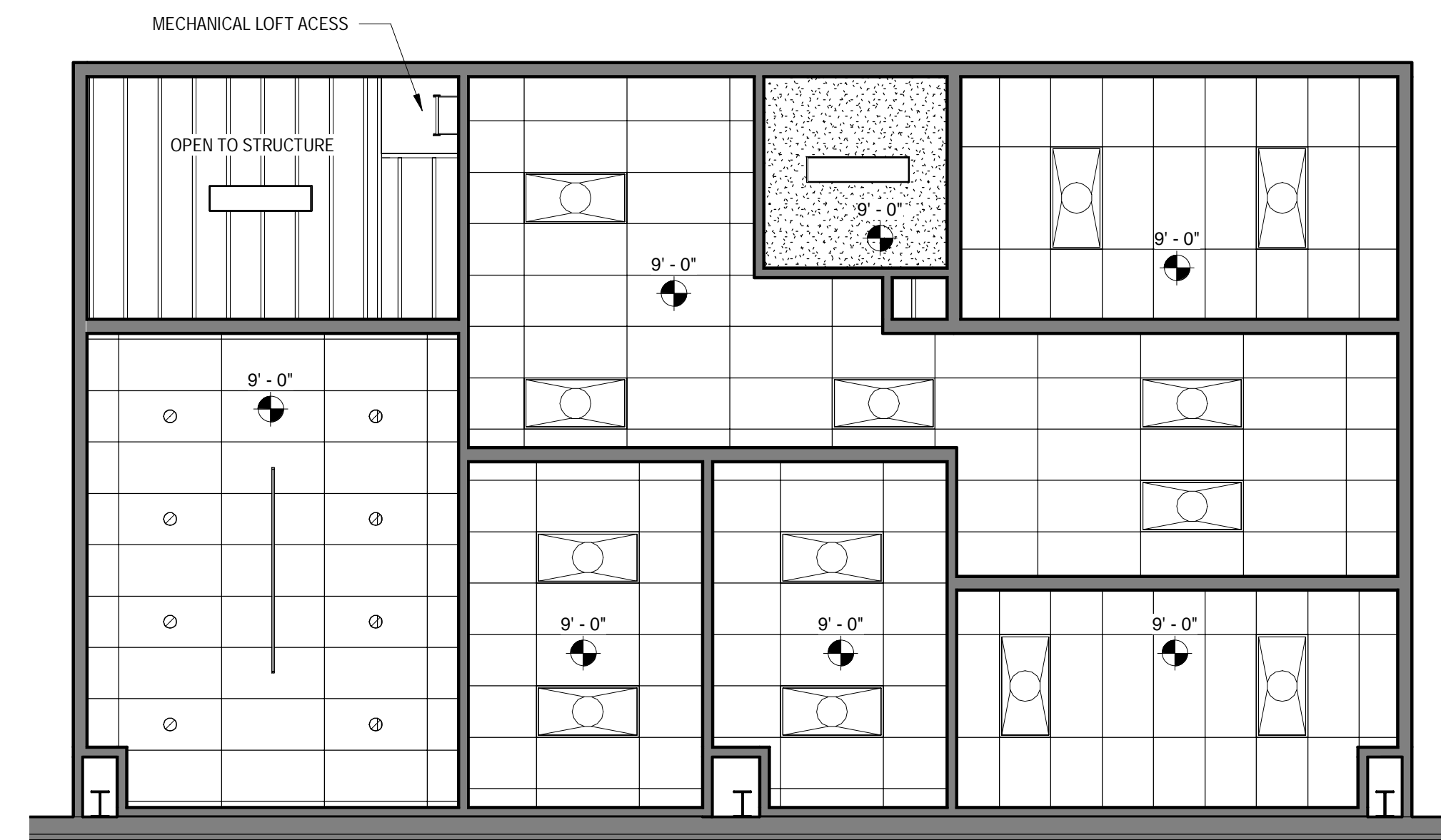
3 REFLECTED CEILING PLAN - 2ND FLOOR A-2.1 SCALE 3/16" = 1'-0"
