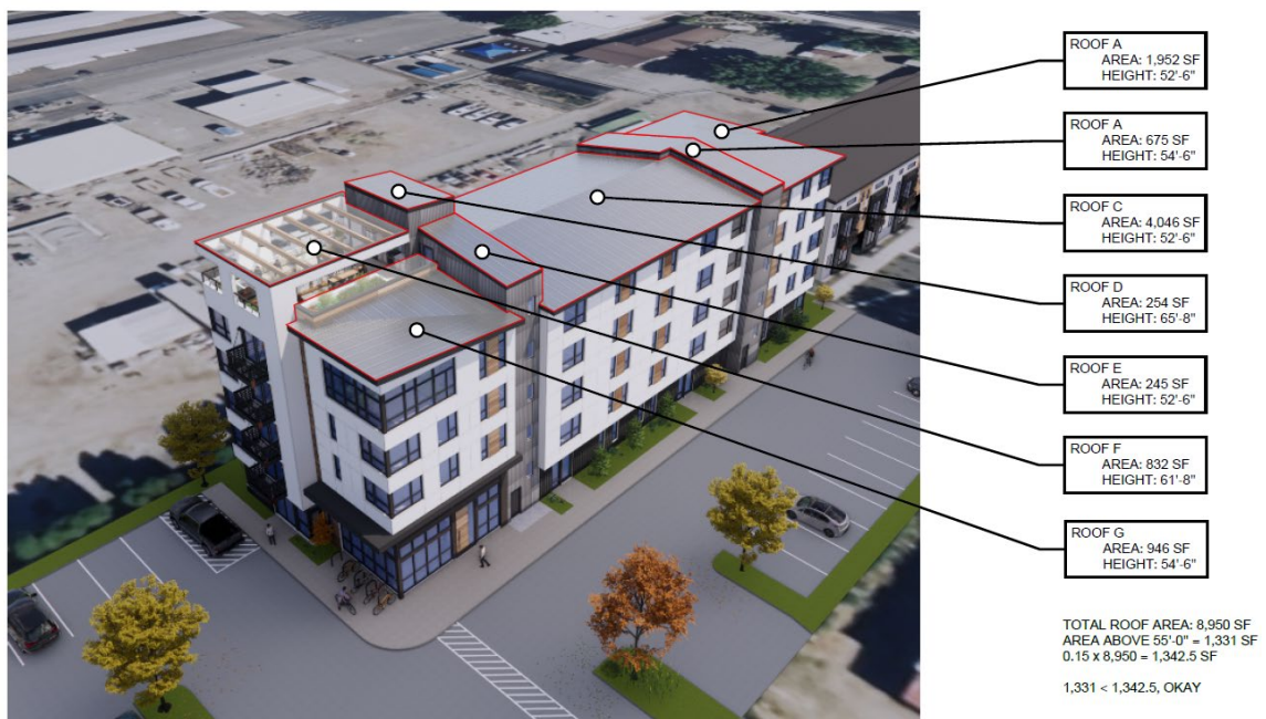
Figure 4 – Roof Plane Analysis
