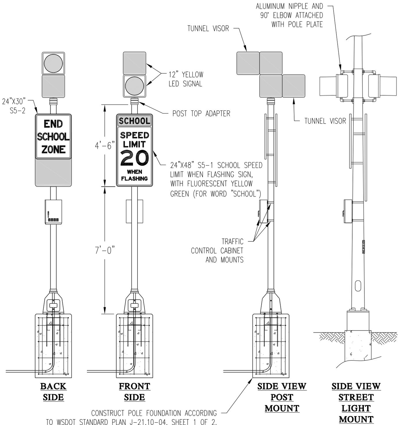
CONSTRUCT POLE FOUNDATION ACCORDING TO WSDOT STANDARD PLAN J-21.10-04. SHEET 1 OF 2. UTILIZE ANCHOR BOLT CAGE FROM MATERIAL LIST. SEE NOTE 1
