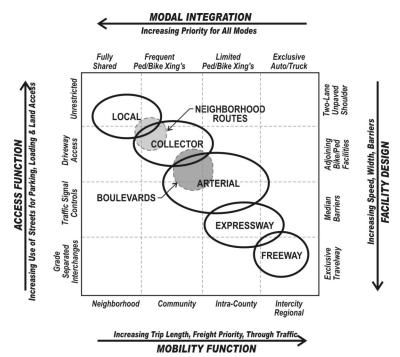
motorized vehicles steadily decreases with higher functional classes. The expressway and freeway facilities typically do not allow pedestrian and bike facilities adjacent to the roadway and any crossings are grade-separated to enhance mobility and safety.
